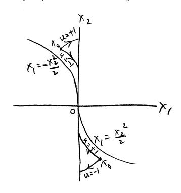
Since  $\dot{x}_2 = \pm 1$ , the curve with the smallest vertical change is time-optimal. In the first case, one can show that this corresponds to u = -1. In the second case, u = +1. Hence, for every  $x_0$  the optimal control is
